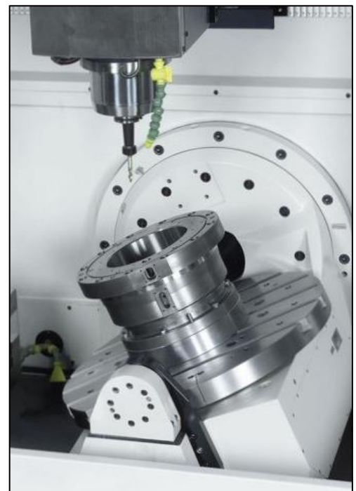
5-axis Machining on a LIT's Spinner CNC machine
