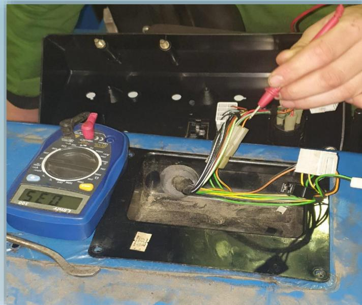
Photo of: Test of PTO Switch.
