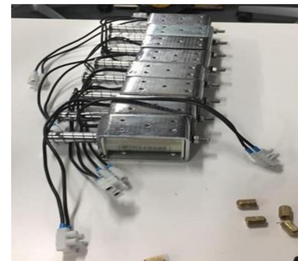
Figure 4: shows the solenoids being Prepared for mounting
