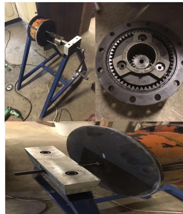
Figure 4. assembly of the planetary gearbox
