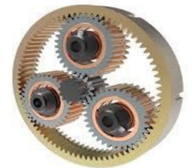
Figure 5. Mechanical motion rectifier within a Planetary gearbox
