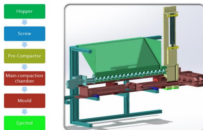
Figure 1: Process Cycle of the Compactor
