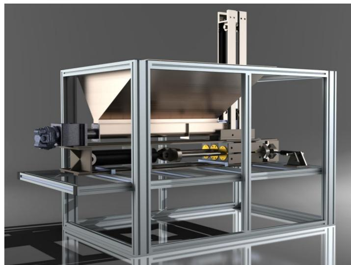
Figure 2: SolidWorks render of swarf compactor
