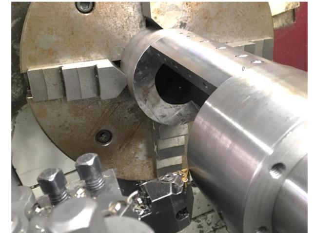
Figure 5: Compaction Barrel in Lathe
